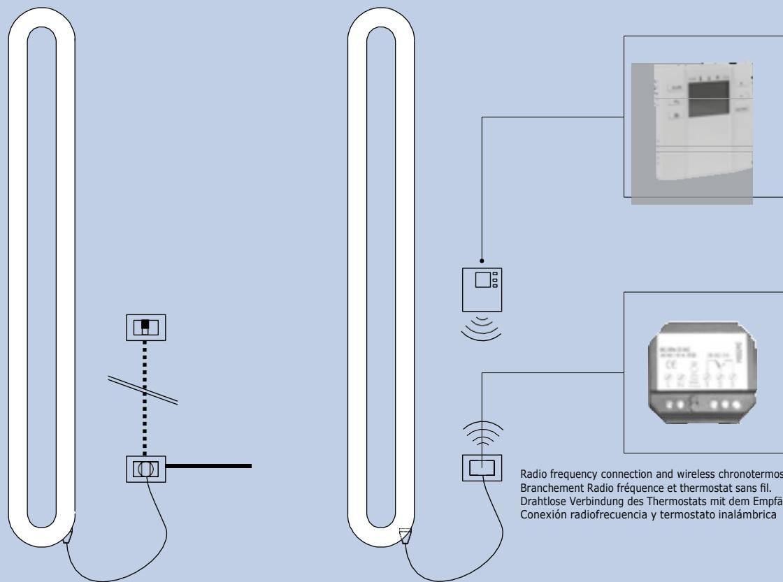
Connection to the electrical socket that is controlled by an ON/OFF switch (not supplied by Antrax)
